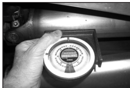
The factory U-joint angle tool, Miller p/n 7336 or C-4244 (bottom, call 800-801-5420 to get one, it's cheap!), makes checking a cinch. A standard magnetic angle finder (top) can also get the job done....
