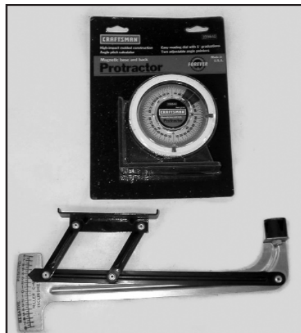
The factory U-joint angle tool, Miller p/n 7336 or C-4244 (bottom, call 800-801-5420 to get one, it's cheap!), makes checking a cinch. A standard magnetic angle finder (top) can also get the job done....
